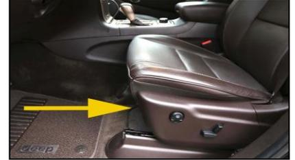
2. Make sure the ignition is off. Locate the rectangular black connector in front, under the driver's seat as shown. Note that there is a tab on each narrow side. These tabs are latch releases.
