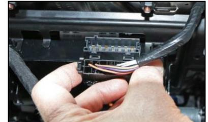
3. Note that the connector is keyed with small protrusions so it cannot go in upside-down. There is one protrusion on the top-side and two protrusions on the bottom-side.
