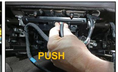
5. Plug the black connector removed in step 2 into the socket on the *SmartStopStart* module. Remember again to align the keyed protrusions with the single protrusion on the top-side so that the connector fits. Press firmly with a thumb on each side until you hear the latches on each side click.
