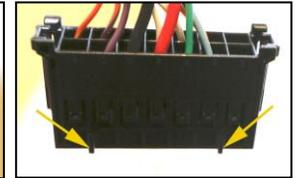
4. Plug the identical black connector from the *SmartStopStart* module into the now empty socket under the seat. Be sure that the side with only one protrusion is on the top so that the connector will plug in.
