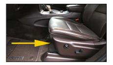
2. Make sure the ignition is off. Locate the rectangular black connector in front, under the driver's seat as shown. Note that there is a tab on each narrow side. These tabs are latch releases.
