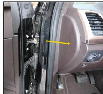
2. With your fingers, pull the weatherstrip away from the door only in the area of this trim panel. The weatherstrip will release when you pull it straight out toward the front of the dashboard.
