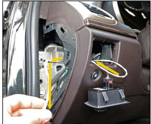
11. Point a flashlight below the OBD2 diagnostic connector under the dashboard, which is just to the right of the parking brake.
