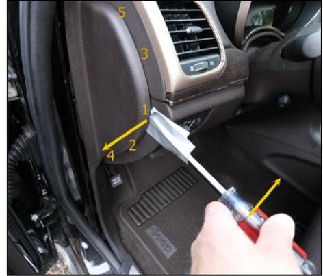
6. Pull the loose panel down to release the A-pillar trim upper catch and then remove the panel.
