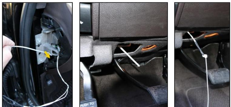
13. Using nail clippers or scissors carefully cut off the zip-tie tail, being very careful not to damage the wires.
