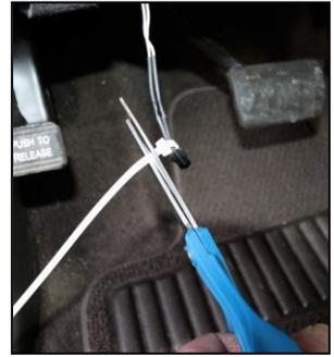
14. Plug the small black connector from the *SmartStopStart* module and the mating connector on the wire from step 12 together until they click. They only fit together in one orientation as shown.
