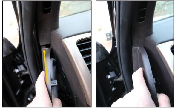
19. Carefully align all 5 tabs and clips with their respective openings on the side of the dashboard.
