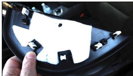
5. Insert the flat blade screwdriver in the seam at the center front of the trim piece ('1' in photo) and pry outward it until it the center clip releases with a click. Then release lower and upper middle clips ('2' and '3'). Lastly release the lower and upper clips ('4' and '5'). Do not attempt to remove the panel yet.
