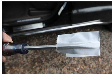
4. Note from this picture of a cover already removed that there are 5 friction-fit trim clips behind the cover that hold it in place. These will need to be released in Step 5.
