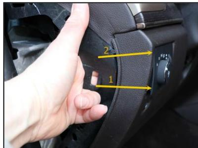
Then push the upper end out ('2' in photo) while pressing at least one of the two spring clips downward on top of the rear of the headlight control panel enclosure until the headlight control panel assembly is released.
