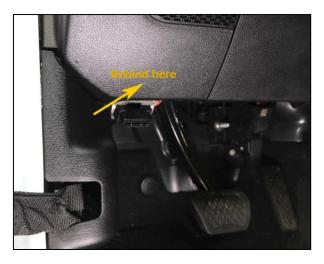
2. Make sure the ignition is off. Using a flashlight, locate the two rectangular black connectors behind the dash <u>as shown in the</u> <u>photo looking up from below the dash</u>.
