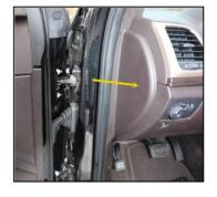
5. Insert the flat blade screwdriver in the seam at the center front of the trim piece ('1' in photo) and pry outward it until it the center clip releases with a click. Then release lower and upper middle clips ('2' and'3'). Lastly release the lower and upper clips ('4' and '5'). Do not attempt to remove the panel yet.
