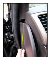
9. Hold the green plug from the SmartStopStart cable in front of the headlamp panel opening as shown.
