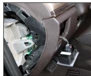
8. Locate the uppermost white socket on the white connector block inside the now open end of the dashboard. This is where the green plug from the SmartStopStart cable will plug-in in Step 9.
