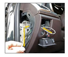
13. Using nail clippers or scissors carefully cut off the zip-tie tail, being very careful not to damage the wires.
