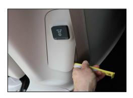
4. Pull the loosened panel out from the bottom with your fingers to release remaining clips and then down to remove.
