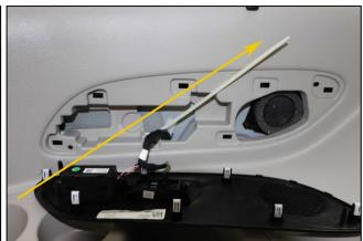
7. Cut two 1" strips of duct tape and tape the **SMALLER** black connector from the long black and red cable supplied to the thin end of the zip tie supplied as shown.
