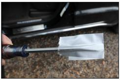
3. Insert the covered flat blade screwdriver in the seam at the lower right of the trim panel (1) and pry outward it until the lower clips release. Do not attempt to remove the panel yet and <u>do not pry at the top</u>.
