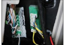
14. Plug the black connector on the red and cable pulled earlier into the black connector from the *Smart*StopStart module. Note that it will only fit in one orientation.
