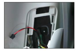
9. Peel the backing off of the Velco strip on back and attach the provided 3-way connector hub in the upper (2) opening as shown:
