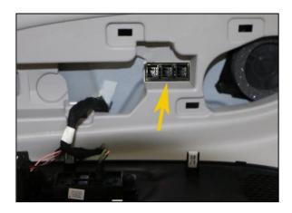
10. Continuing at the black panel removed at the upper opening (2), press the tab on the 3-wire connector at the back of the USB module and pull the connector out. Then reinsert this same connector in the leftmost position of the 3-way connector hub until it clicks.
