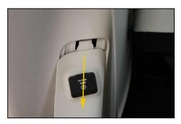
5. Insert the covered flat blade screwdriver in the seam at the top of the black 3<sup>rd</sup> row passenger side trim panel (2) and pry outward it until the upper clips release. Then simply pull the complete panel straight out toward you with your fingers until the remaining clips release.
