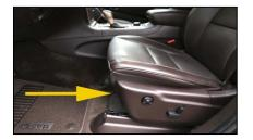
2. Locate the rectangular black connector in front, under the driver's seat as shown. Note that there is a tab on each narrow side. These tabs are latch releases.
