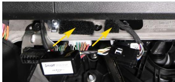
6. Firmly press the SmartStopStart module body and loose connector onto their respective Velcro patches. Do not pull them off again to reposition now, as it will take a few hours for the adhesive to hold tight.
