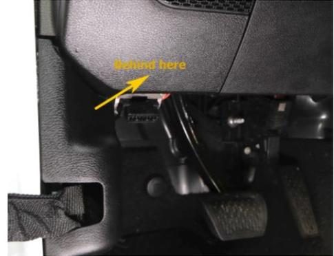
2. Make sure the ignition is off. Using a flashlight, locate the two rectangular black connectors behind the dash **as shown in the photo looking up from below the dash.**
