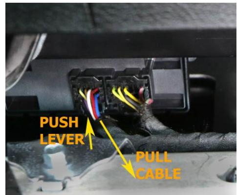
3. Plug-in the identical 8-wire connector with the longer cable from the SmartStopStart module into the now empty connector slot until it clicks. Note the orientation of the connector must be the same as in step 2 for it to fit.
