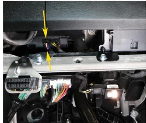
Using the index finger of your left hand, FULLY depress the lever (tab) in the middle of the connector (on the opposite side of the trapezoid shape). At the same time gently tug on the cable with your right hand until it releases.
