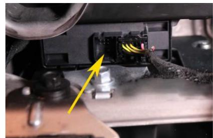
4. Plug the black 8- wire connector unplugged earlier from the vehicle into the socket on the shorter cable from the SmartStopStart module.
