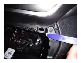
4. Press the tab (see yellow arrow) on the connector behind the panel and pull the connector body away to release it.
