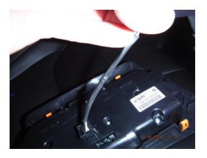
6. Plug the removed cable into the SmartStopStart module.
