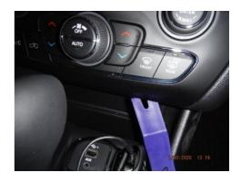
3. Use the flat curved pry bar to pry the <u>upper</u> right of the panel until it pops. Then repeat for the upper left until the panel is completely released. (The photo shows the tool pointing to the area to pry on the right with the panel already removed.)
