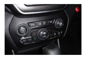
2. Make sure the ignition is off. Use the angled plastic pry bar included in the kit (color may vary) to pry the <u>lower</u> end of the bezel on the right as shown until it pops. A slight twisting action should pop the hidden fastener. Then repeat on the left side.
