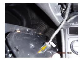
5. Plug the SmartStopStart module into the connector on the panel.
