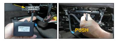
5. Plug the black connector removed in step 2 into the socket on the *Smart*StopStart module. Remember again to align the keyed protrusions with the single protrusion on the top-side so that the connector fits. <u>Press</u> firmly with a thumb on each side until you hear the latches on each side click.
