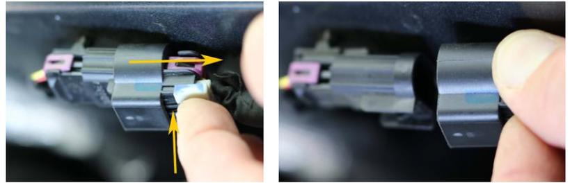
5. Plug the module in between the two separated connector halves in the vehicle.
