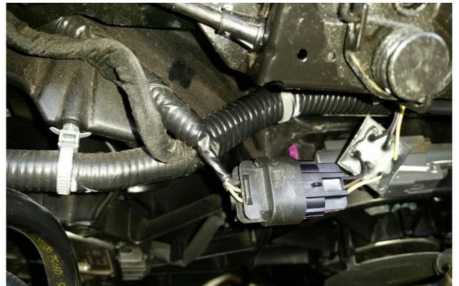
7. Any excess wiring slack can be taken up with a small cable tie provided.
