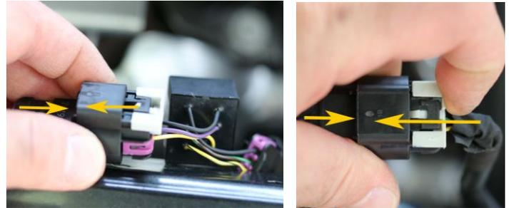
6. The installed module shown in the photo. The module can be tie-wrapped to a nearby cable with a long tie-wrap provided (not shown). The tie-wrap excess can be trimmed.
