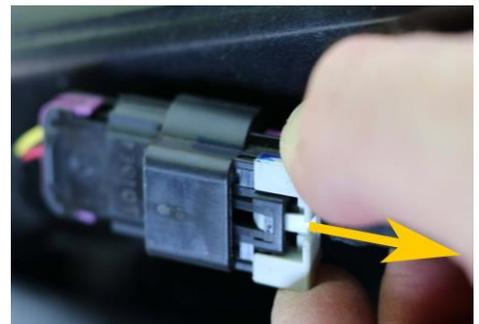
4. Depress the black plastic lever in the center between the gray arms **FIRMLY** with while pulling the connector shells apart. The connector halves will separate.
