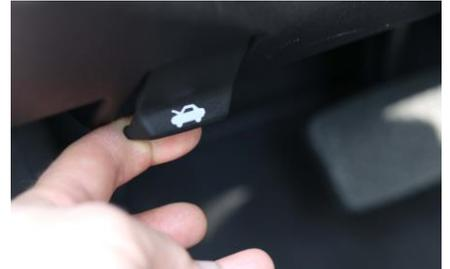
Then, from the front of the vehicle, find the secondary hood release handle. The handle is under the front edge of the hood near the center. Push the handle to the right and raise the hood.
