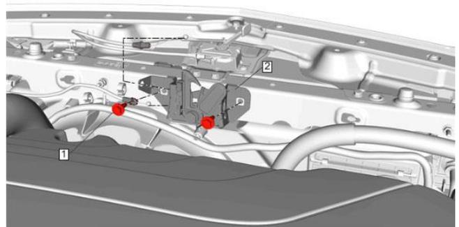
3. Slide the gray plastic locking piece on the connector about 1/8" (3 mm) away from the connector body until it stops. (Some vehicles may not have the gray locking piece, in that case skip to step 4).
