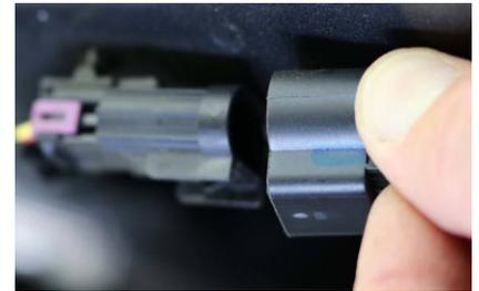
6. Plug the module in between the two separated connector halves in the vehicle.
