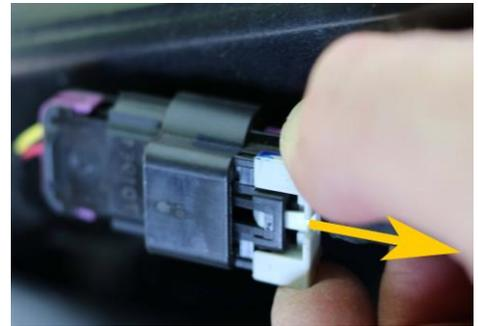
5. Depress the black plastic lever in the center between the gray arms FIRMLY with while pulling the connector shells apart. The connector halves will separate. On 2018 models (shown) the black lever is in the center between the gray arms of the locking piece. On 2019 models the black lever is above the red locking piece.
