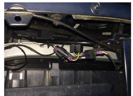
8. Any excess wiring slack can be taken up with a small cable tie provided.
