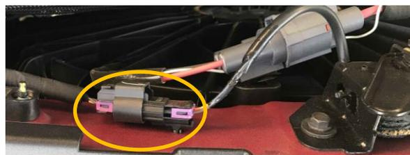
4. Slide the gray plastic locking piece on the connector about 1/8" (3 mm) away from the connector body until it stops. (**NOTE 1:** Some vehicles may not have the gray locking piece, in that case skip to step 4). (**NOTE 2:** On 2019 models slide the red locking piece to the right).
