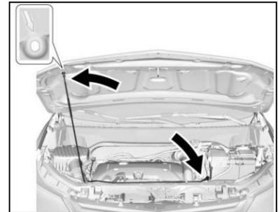
3. Remove the UPPER top front cover over the radiator and hood latch. To remove the front cover, the plastic fasteners must be removed as shown to the right. The number of fasteners and placement may vary slightly between vehicles.
