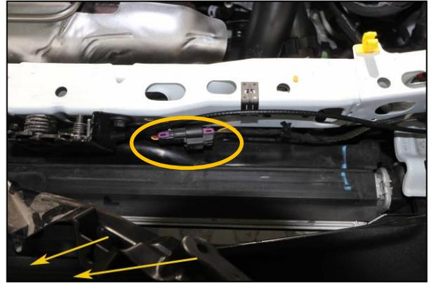
6. Slide the gray plastic locking piece on the connector about 1/8" (3 mm) away from the connector body until it stops. (Some vehicles may not have the gray locking piece, in that case skip to step 7). **(NOTE: On 2019 models slide the red locking piece to the right).**
