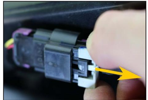
7. Depress the black plastic lever in the center between the gray arms FIRMLY with while pulling the connector shells apart. **On 2018 models (shown) the black lever is in the center between the gray arms of the locking piece.** **On 2019 models the black lever is above the red locking piece.** The connector halves will separate.
