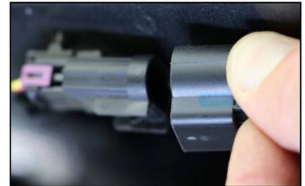
8. Plug the module in between the two separated connector halves in the vehicle.
