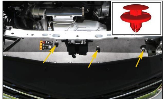
4. Remove the fasteners shown from the LOWER top front cover over the radiator and hood latch.
