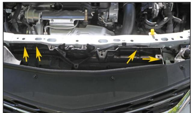
5. The right side of the lower plastic cover should now be lifted up and out of the way. Locate the black and purple plastic connector above the radiator and beside the hood latch. **(NOTE: On 2019 models the connector is black and red).**
