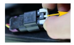
4. Depress the black plastic lever. FIRMLY with while pulling the connector shell to the right.
