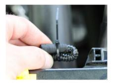
7. Use supplied large tie-wrap to affix the module in place on the <u>side of the rail</u> above the radiator. Run the wire tie in the space between the criss-crossed wires on module and around the entire rail. <u>WARNING:</u> DO NOT mount the module or its connectors on the top of the rail. If you do, they will interfere with hood closing and potentially damage (dent) the hood when it is closed.
