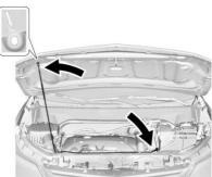
2. Look at the front of the vehicle under the hood. Locate the black, purple and grey plastic connector in the center near the hood latch on the side of the rail above the radiator. (NOTE: On 2019 models the connector is black and red).
