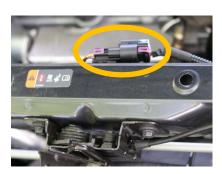
3. Slide the gray plastic locking piece on the connector about 1/8" (3 mm) to the right until it stops. (NOTE: On 2019 models slide the red locking piece to the right).
