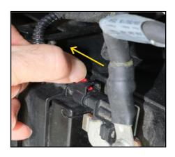
7. Depress the black plastic lever (which is part of the connector body, just to the left of the red tab) FIRMLY with while pulling the connector shell to the left.
