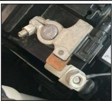
6. Locate the <u>connector with 2 wires</u> <u>attached directly to the negative battery post</u>. Slide the red plastic locking piece on the connector about 1/8" (3 mm) to the left until it stops.
