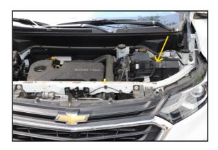
4. Locate the battery negative terminal with the battery sensor.
