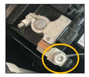
5. Locate the <u>connector with 2 wires attached to the negative battery post</u>. Slide the red plastic locking piece on the connector about 1/8" (3 mm) to the left until it stops.
