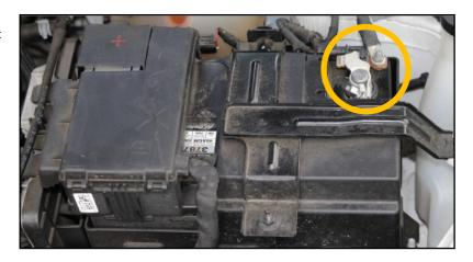
4. Remove the larger (13mm) nut at the negative battery terminal (counterclockwise) but DO NOT take the terminal with the thick wire off of the stud. Place the round silver ring terminal with the black wire from the SmartStopsStart GMII module over this threaded stud. Screw back on the 13mm nut by hand and then and tighten the nut firmly clockwise with a 13mm wrench.
