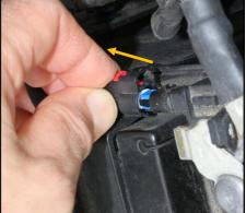
7. Now plug the SmartStopStart GM II module in between each of the two separated connector halves in the vehicle.
