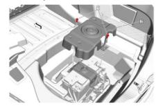
3. Locate the battery negative terminal with the battery sensor. Your battery may appear different than the photo.
