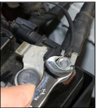
6. Locate the connector with 2 wires attached directly to the negative battery post. Slide the red plastic locking piece on the connector about 1/8" (3 mm) to the left until it stops.
