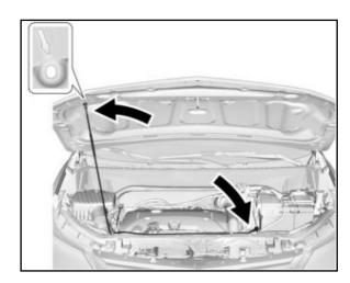
3. Locate the battery. The battery is under the hood on the driver's side. The battery may differ from the photo.
