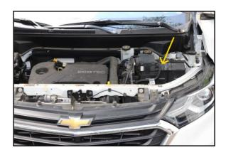
4. Locate the battery negative terminal with the battery sensor.
