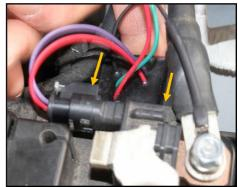
10. Use a supplied tie-wrap to secure the hanging connector body to a nearby cable.
