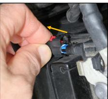
8. Now plug the SmartStopStart GM II module in between each of the two separated connector halves in the vehicle.
