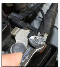
5. Locate the connector with 2 wires attached to the negative battery post. Slide the red plastic locking piece on the connector about 1/8" (3 mm) to the left until it stops.
