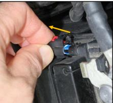
7. Now plug the SmartStopStart GM II module in between each of the two separated connector halves in the vehicle.
