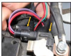
9. Use a supplied tie-wrap to secure the hanging connector body to a nearby cable.
