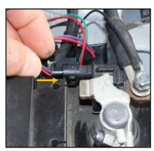
8. Apply the supplied Velcro patch to the rear of the battery outer black plastic box. Press the module onto the Velcro patch.
