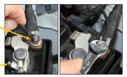
5. Locate the connector with 2 wires attached to the negative battery post. Slide the red plastic locking piece on the connector about 1/8" (3 mm) to the left until it stops.
