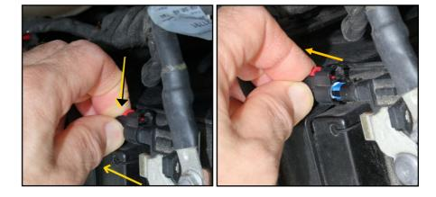
7. Now plug the SmartStopStart GM II module in between each of the two separated connector halves in the vehicle.
