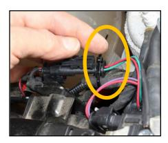
11. Installation is complete! Auto-stop will now be disabled after the vehicle is locked and not driven one time for at least 8 consecutive hours (typically overnight).
