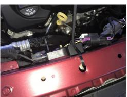
7. Any excess wiring slack can be taken up with a small cable tie provided.
