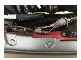
3. Slide the gray plastic locking piece on the connector about 1/8" (3 mm) away from the connector body until it stops. (Some vehicles may not have the gray locking piece, in that case skip to step 4). (NOTE: On 2019 models slide the red locking piece).
