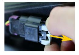
4. Depress the black plastic lever FIRMLY while pulling the connector shells apart.
