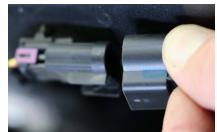
5. Plug the module in between the two separated connector halves in the vehicle.
